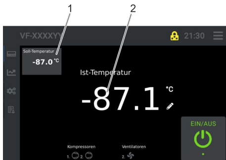
Fig. 125: Cooling chamber temperature set point icon
